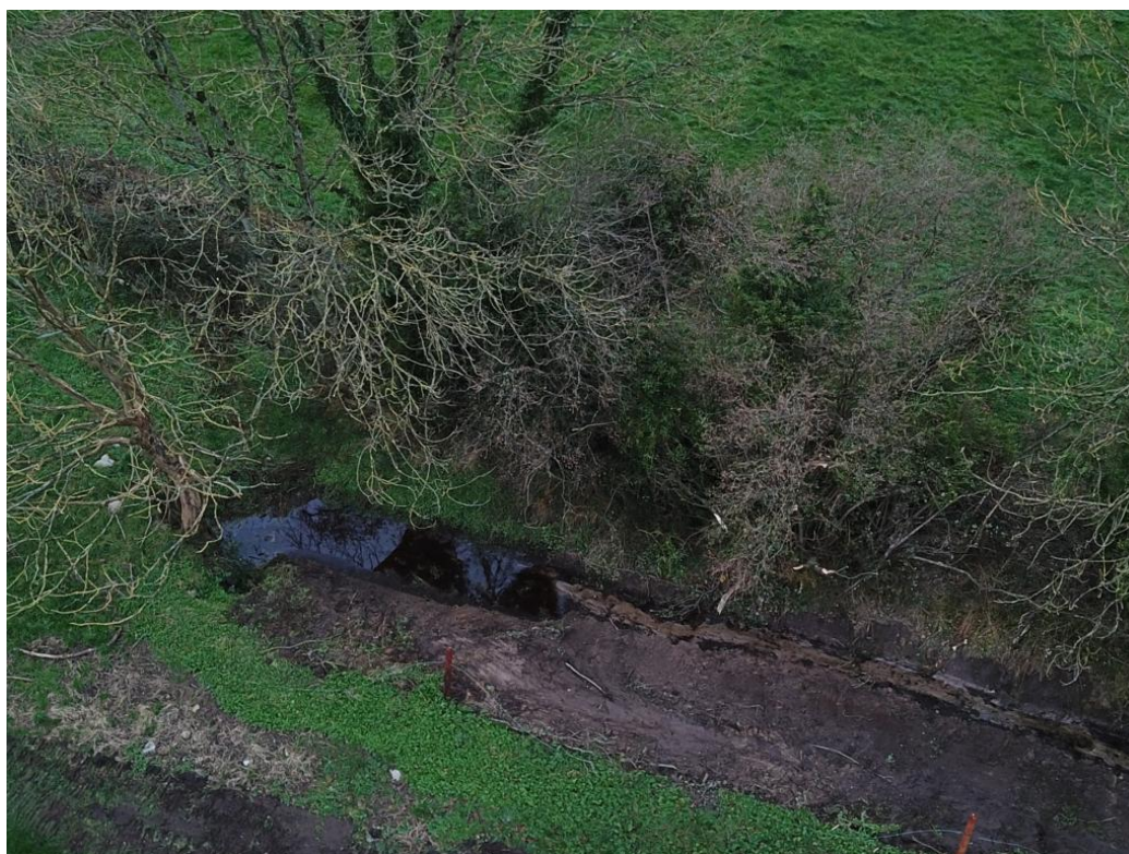
Plate 5: Aerial view of water feature MP4A (swallow hole to south of IP1) after dye release -no breakthrough was observed on the day
