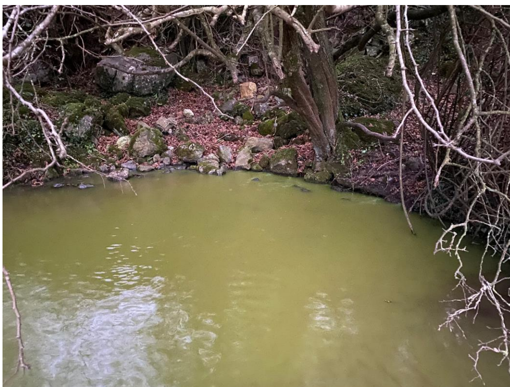
Plate 8: Ground view of main spring feature (MP1/ IP4) after dye release at IP1 (14:41hrs) -Estimated breakthrough at 16:37hrs at IP4 above
