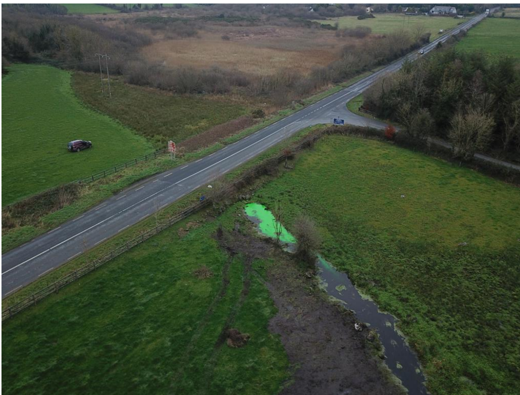
Plate 2: Aerial view of Fluorescein dye release (injection at 14:41hrs north of road)
