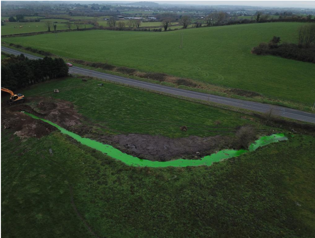
Plate 3: Aerial view of Fluorescein under flow conditions, South towards swallow hole (IP1)
